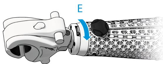
To remove the terminal device, slide the wrist button slider back to the "Open" position and then pull out the device.
