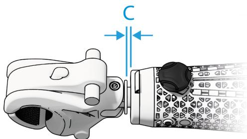
At the second click (fully inserted), the device will be held so that it can't pull out, and so that it can't rotate either. This is the Fully Locked mode. In this mode, the insert can be tightened further or unscrewed by twisting the terminal device.
