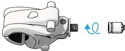
To attach the device to your Hero Flex, press the wrist button (**A**) and, at the same time, push the terminal device into the opening in the wrist (**B**):
