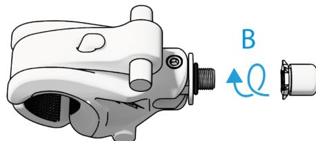
By adjusting how tightly the insert is screwed in, you can adjust how easily the tool will rotate in the wrist. If you don't compress the O-ring at all, the device will "freewheel". If the O-ring is very compressed, the tool will stay in place until you manually rotate it.
